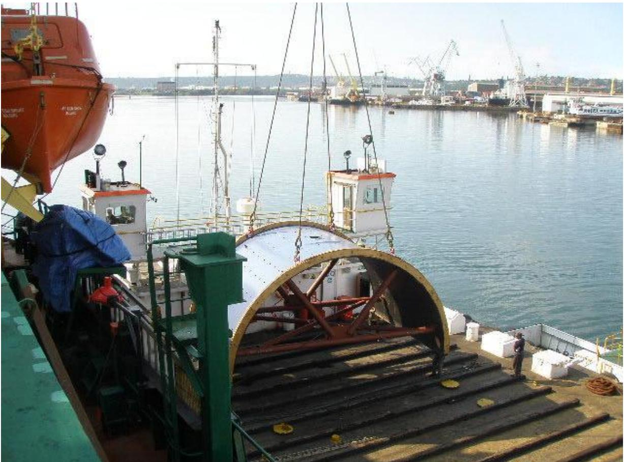
**Figure 4 – Ball mill shells being transferred from Singapore to Manila**
